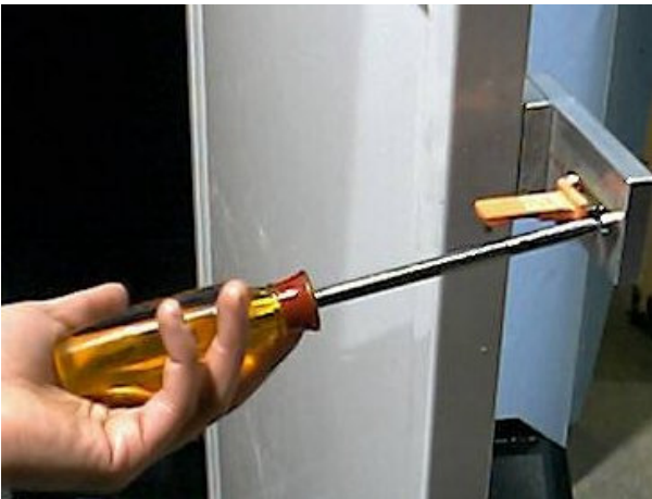
FIG. 12- ADJUST INTERLOCK KEY TAB IF NECESSARY (MAY NOT BE SAME AS PICTURED)
