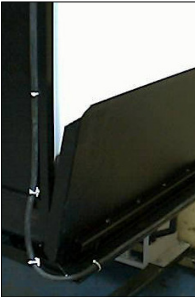
FIG. 14- FASTEN CABLE TO SAFETY PLATE USING STRAPS
