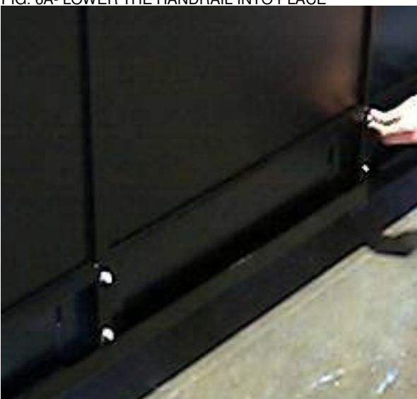
FIG. 6B- BOLT HANDRAIL TO CARRIAGE
