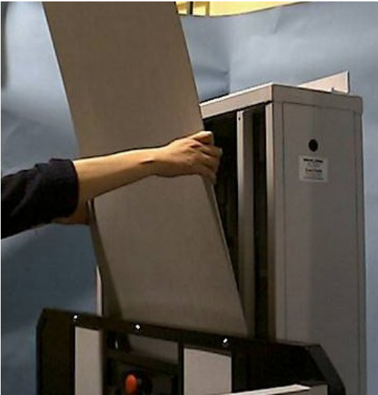
FIG. 19- REMOVING FRONT COVER PANEL
