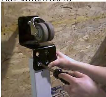
FIG.3-BOLT CASTOR TO THE BASEFRAME
